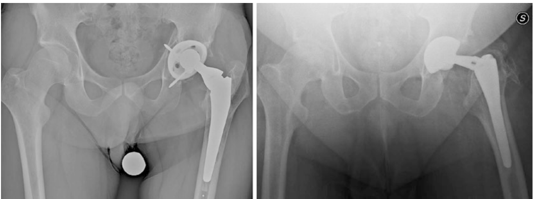
Fig. 8.4 Ti proximal modularity may face disassembling (left image) and neck failure (right image): disassembling occurred after a trauma 20 years after the implantation.
